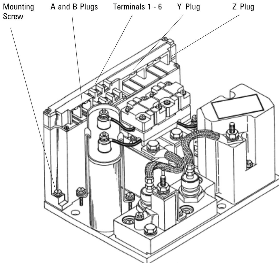
Disconnect the battery and discharge the capacitor. Measure ohms through the capacitor using the R x 10,000 scale. Meter should read zero and then swing slowly to above 100,000 ohms. Replace the capacitor if above reading is not obtained.
