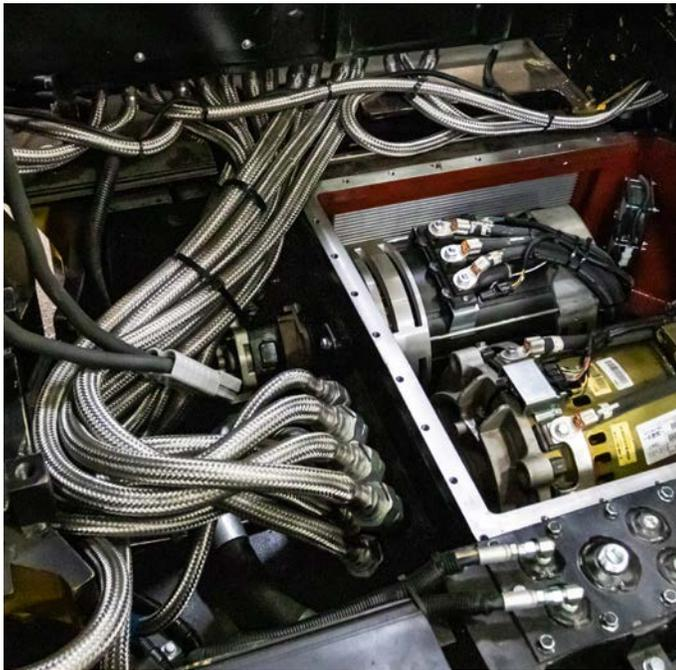
**FLEXIBLE CONDUIT (FC) CABLES** house regular cabling, which is sealed to ensure safe use in an EX-rated environment. The FC Cable provides flexibility and space saving.
