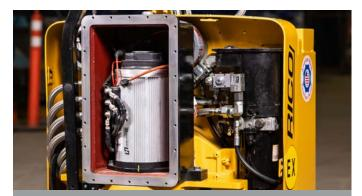
**DRIVE, PUMP AND ELECTRICAL ENCLOSURES** house only electrical components and are approved to be included on EX-rated lift trucks. All RICO enclosures have been tested for approval in an EX-rated environment by FM Global.
