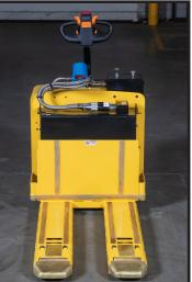
The exposed components on the perimeter of the truck, including forks, are protected with brass and aluminum. This helps to **PREVENT ELECTRICAL** FRICTION SPARKS, which can ignite the hazardous environment. Both brass and aluminum are alloys which reduce heat and the possibility of sparking.
