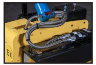
Regular cabling is sealed into a **FLEXIBLE CONDUIT (FC) CABLE**, ensuring safety, making them liquid and gas tight. The FC Cable provides flexibility and space saving.
