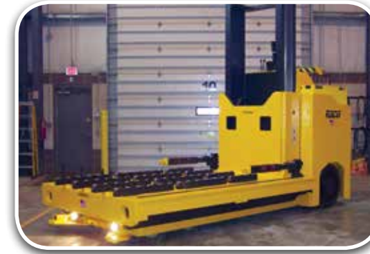
80K Front Push w/Docking Camera & Pendant Control
