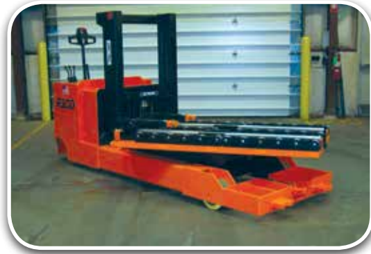
10K Rotating Positioning Table Walk Behind
