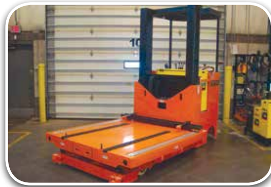
30K Front Push w/Low Profile Roller Rider
