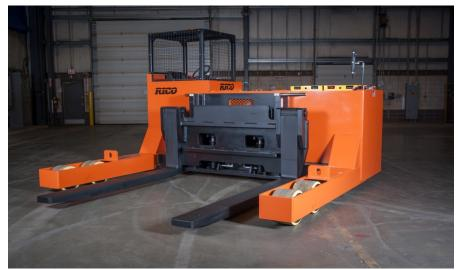
BPR-Rico Manufacturing is used to unique challenges customers bring them. When representatives of the textile industry in China called looking for better ways to transport fabric stacks, Rico designers went to work. The fabric, by nature, does not stack in neat blocks and can be awkward in shape. They could also be up to 35,000lbs bundles creating an unstable and unsafe load if not supported properly during transporting.
