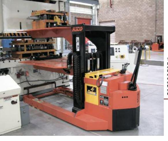
This two-tier die cart placed near the press aids in quick die change by serving as a staging rack for a die waiting to run and at the same time can hold a die removed from the press. The setup saves on travel time for die retrieval.
