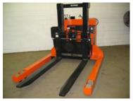
The walkie style pallet stacker is the most commonly used of all electric powered pallet stackers. Pallet stackers are similar in design and function to <u>counterbalance lift trucks</u> but have many additional functions and advantages.
