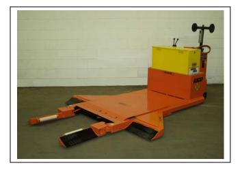
The RICO Vehicle Mover is the answer to the need for moving disabled vehicles quickly off or onto an assembly line. This custom designed Vehicle Mover has the lifting capacity of 20,000 lbs. and a pulling capacity of 27,000 lbs. Specially designed controls to disengage the air brakes of the FMTV A1 R have been installed on the RICO Vehicle Mover. This will allow the truck to roll freely while operating the RICO Vehicle Mover.
