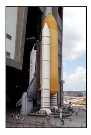
Each space shuttle has SRB's designed to produce the main thrust to lift the space shuttle off the pad and up to an altitude of about 150,000 feet, or 24 nautical miles. The two SRB's carry the entire weight of the external tank and orbiter. The SRBs are the largest solid-propellant motors ever flown and the first designed for reuse. Each is 149.16 feet long and 12.17 feet in diameter.
