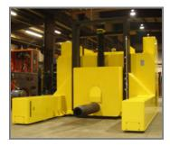
Coil ram lift is precisely controlled via a linear ball screw and an electric motor coupled to a gear box. Each of the two steer-drives are electrically actuated and designed to be controlled independently through the use of an electronic Ackerman steering system. A traditional mechanical tie-bar is no longer required.
